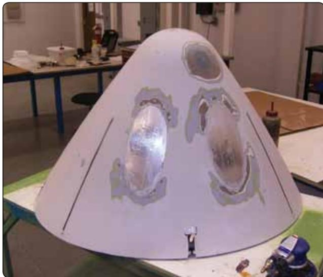
**Figure 7-21.** Damage to radome honeycomb sandwich structure.
