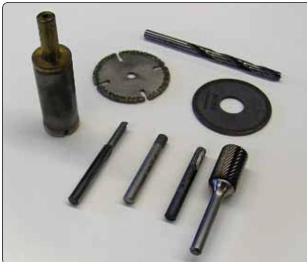
Figure 7-86. Drilling and cutting tools for composite materials.
