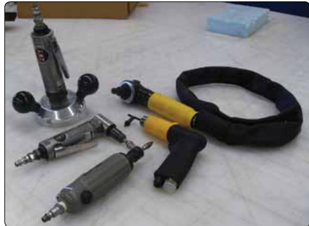
**Figure 7-32.** Air tools used for composite repair.
