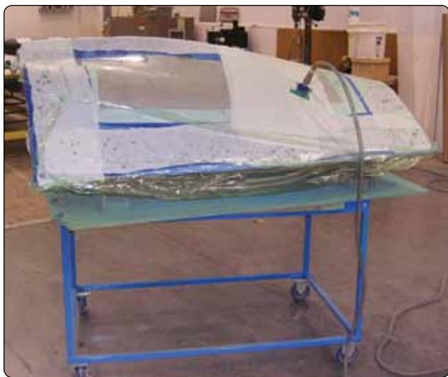
Figure 7-52. Envelope bagging of repair.
