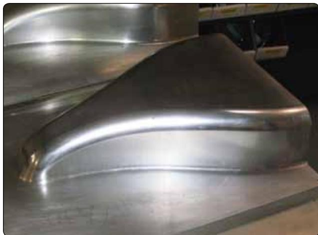
**Figure 7-34.** A mold of an inlet duct.
