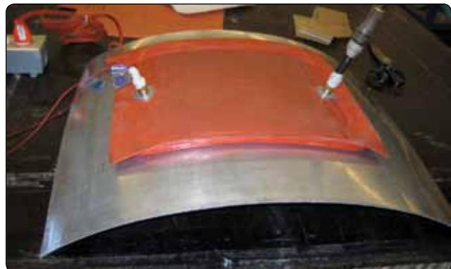
**Figure 7-37.** Self-sealing vacuum bag with heater element.
