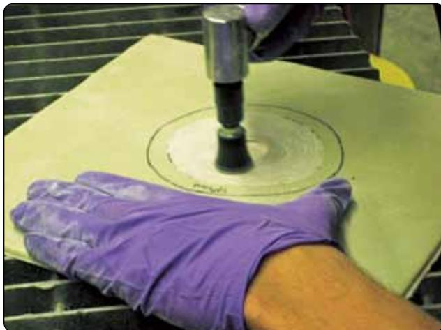
**Figure 7-58.** Taper sanding of repair area.
