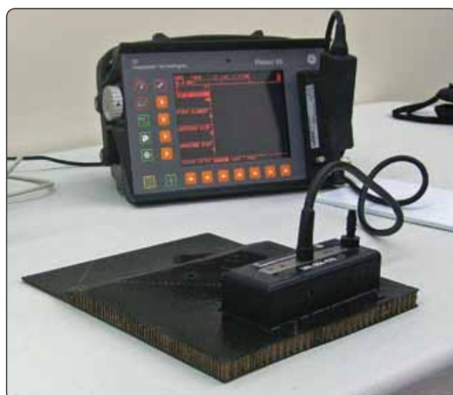
Figure 7-28. Phased array testing equipment.
