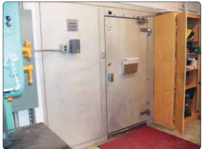
Figure 7-44. Walk-in freezer for storing prepreg materials.
