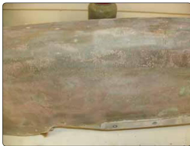
**Figure 7-8.** Copper mesh lightning protection material.
