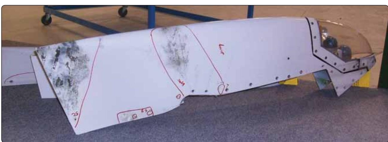
**Figure 7-22.** Erosion damage to wingtip.
