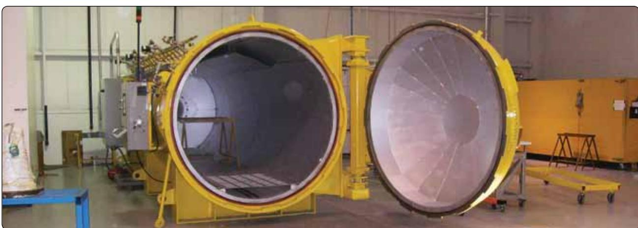
**Figure 7-39.** Autoclave.
