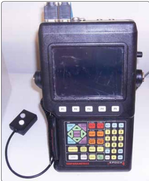
Figure 7-26. Pulse echo test equipment.
