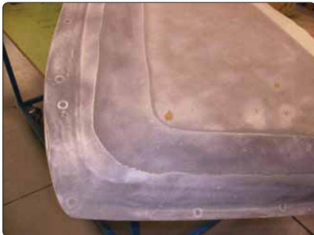
**Figure 7-9.** Aluminum mesh lightning protection material.
