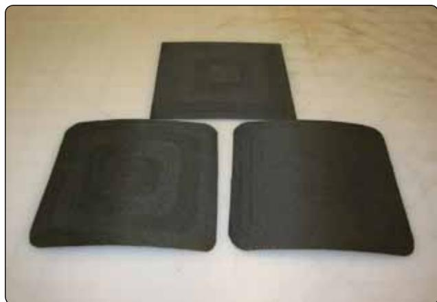
**Figure 7-73.** Precured patches.
