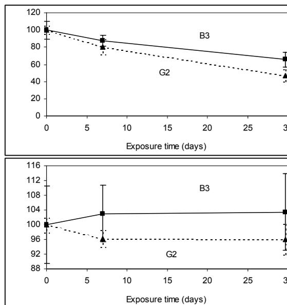
These results confirm basalt's better resistance to alkali, compared to E-glass.
