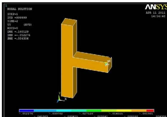
Displacement Solution For Beam-Column Joints As Per Code Is 456: 2000 For The Load of 49.5 kN
