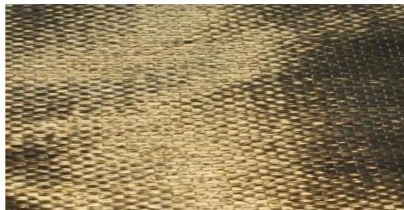
**Fig 1. Basalt Fibre**
