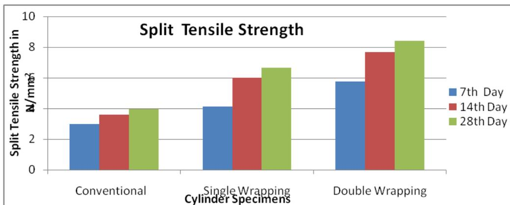
Fig 5. Comparison of Split Tensile strength
