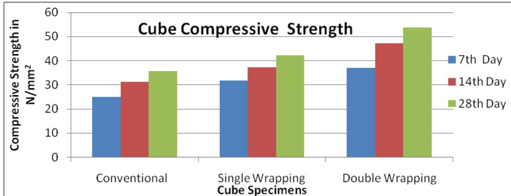
Fig 4. Comparison of Compressive strength
