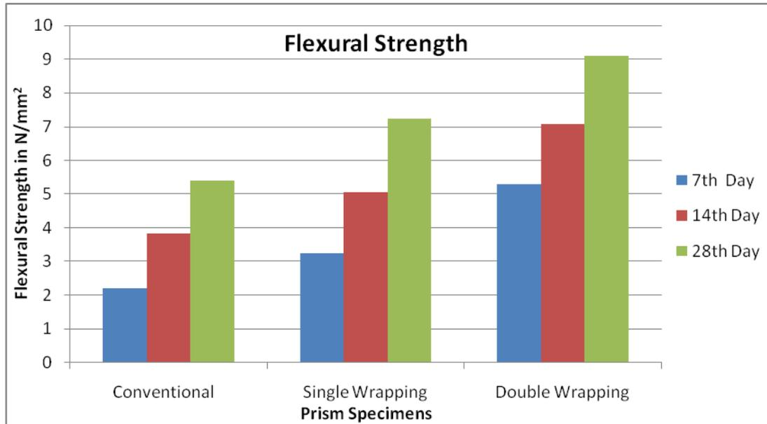
**Fig 6. Comparison of Flexural strength**
