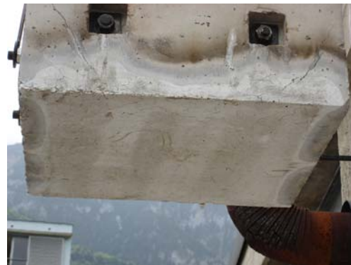
Fig. 6. Spalling of the surface previously heated – normal concrete and fiber reinforced concrete
