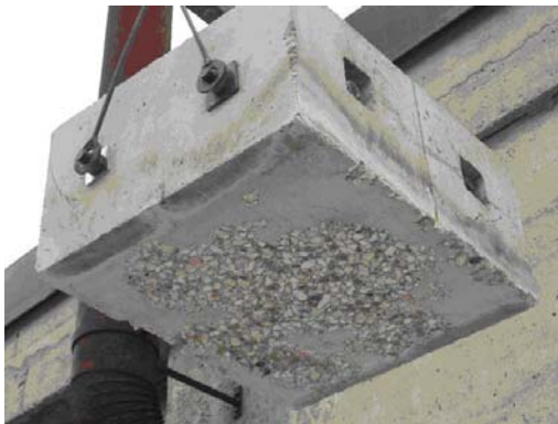
Fig. 6. Spalling of the surface previously heated – normal concrete and fiber reinforced concrete
