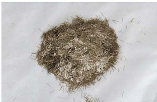
*Figure 1* : Basalt fibre
