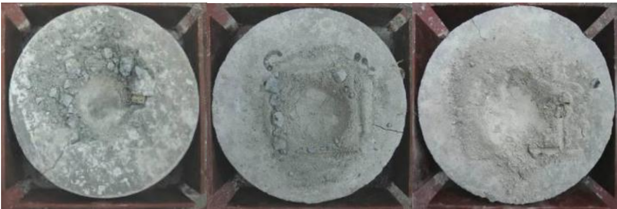
Fig. (5). Basalt fiber-reinforced concrete failure pattern.
