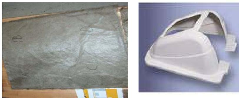
Picture 4 Basalt fiber reinforced polypropylene thermal plasticity composites mat and sample
