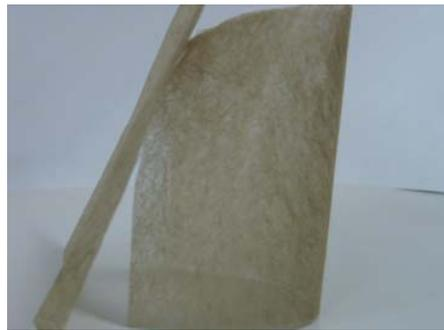
Picture 3 Basalt fiber surface mat
