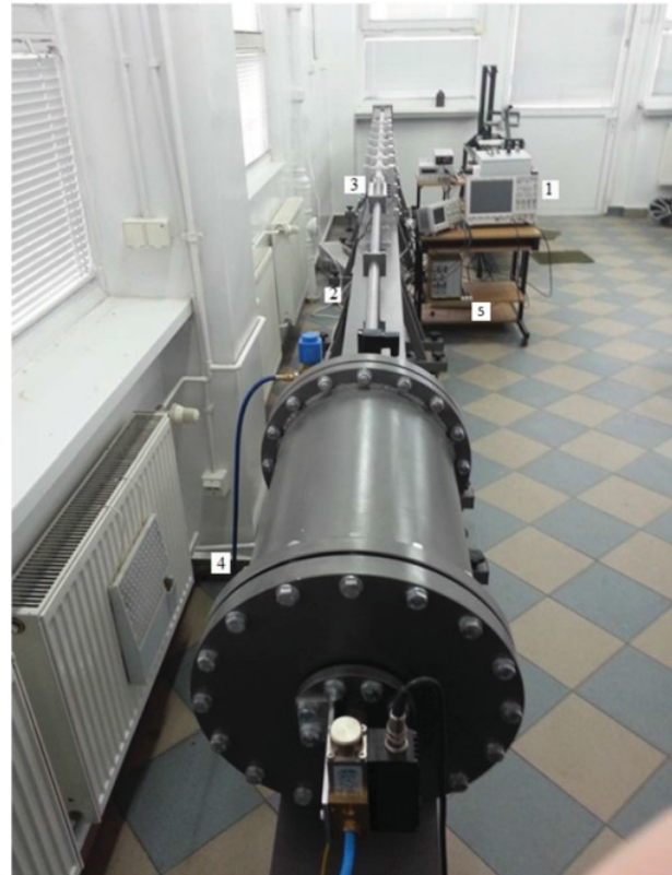
Figure 1. Split Hopkinson bar arrangement applied in the dynamic tests. 1 – digital oscilloscope, 2 – base, 3 – steel bars, 4 – pressure tank, 5 – tensometer bridge.
