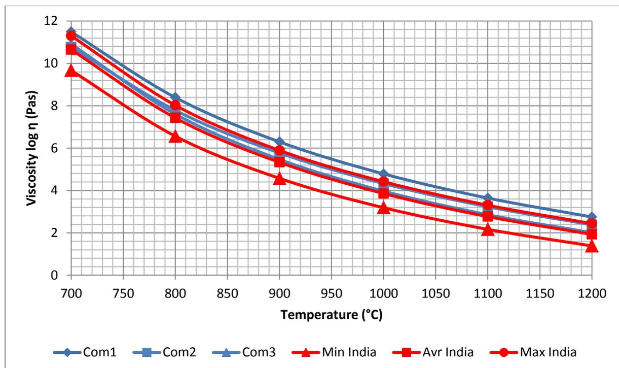
Fig. 6: Plot for viscosity vs Temperature of different basalt raw materials (commercial basalt fibers in blue and Indian Basalt in red)
