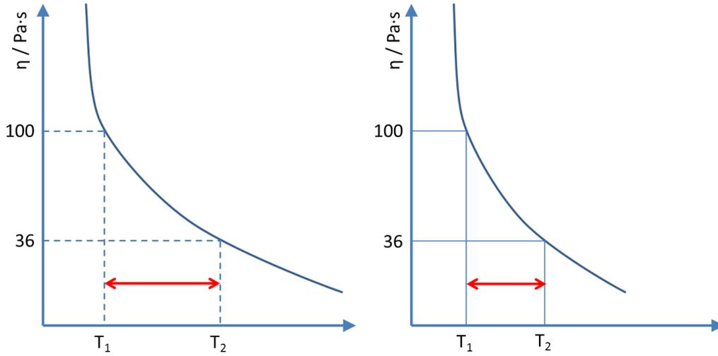
Fig 3. Plot of viscosity vs. temperature. Examples of melts with wide (left) and narrow (right) temperature interval of fiberization and their dependency with the viscosity.
