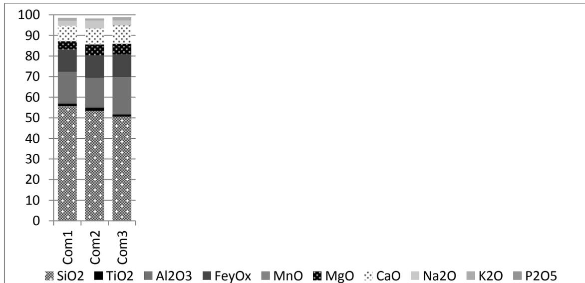
Fig. 5: chemical composition of three raw materials for fiberization of basalt fibers [6].
