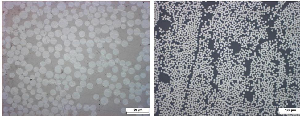
Figure 3: Reflecting microscope picture of a polished section of a basalt-epoxy test specimen (left) and a carbon-epoxy specimen (right)
