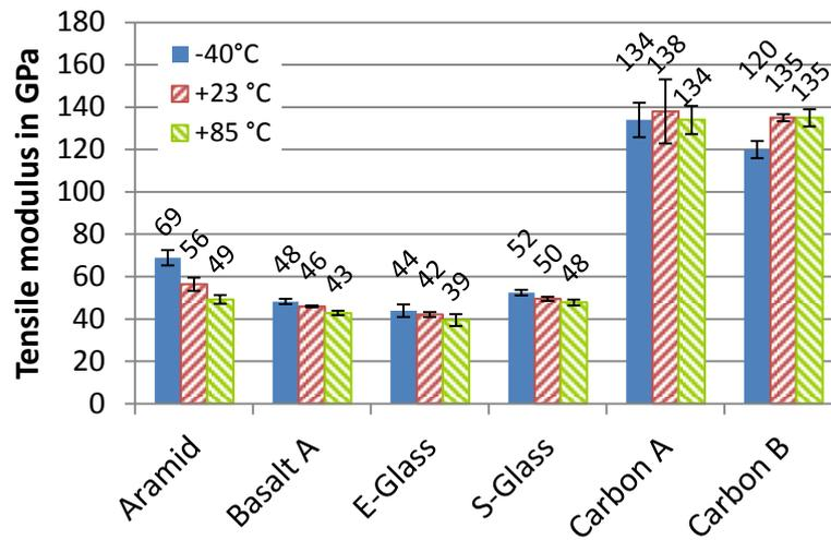
Figure 9: Tensile modulus of different tested polymer fiber composites with epoxy matrix at -40 °C, +23 °C and +85 °C
