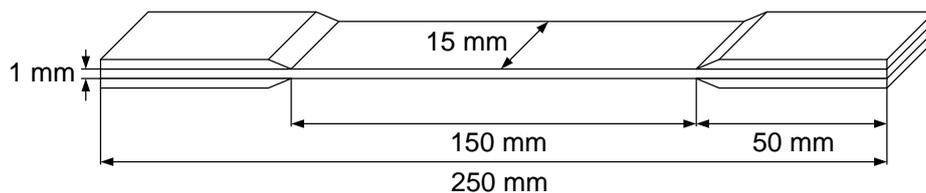
Figure 2: Dimensions of the tensile test specimens
