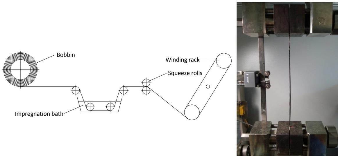
Figure 4: Left: Manual winding device to impregnate rovings according to German standard DIN 65382 [8]; right: tensile test of an impregnated roving in the testing machine
