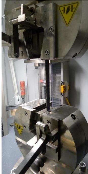
Figure 5: Tensile test of flat unidirectional polymer fiber composite test specimen without temperature chamber
