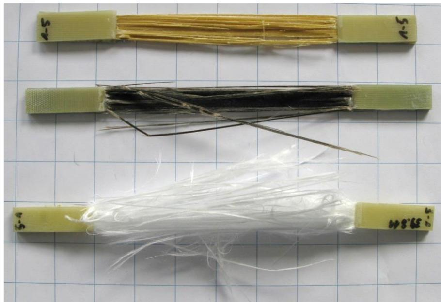
Figure 10: Failure of tensile test specimens aramid-, basalt-, and S-glass composite (from top to bottom) by fiber splitting at -40 °C
