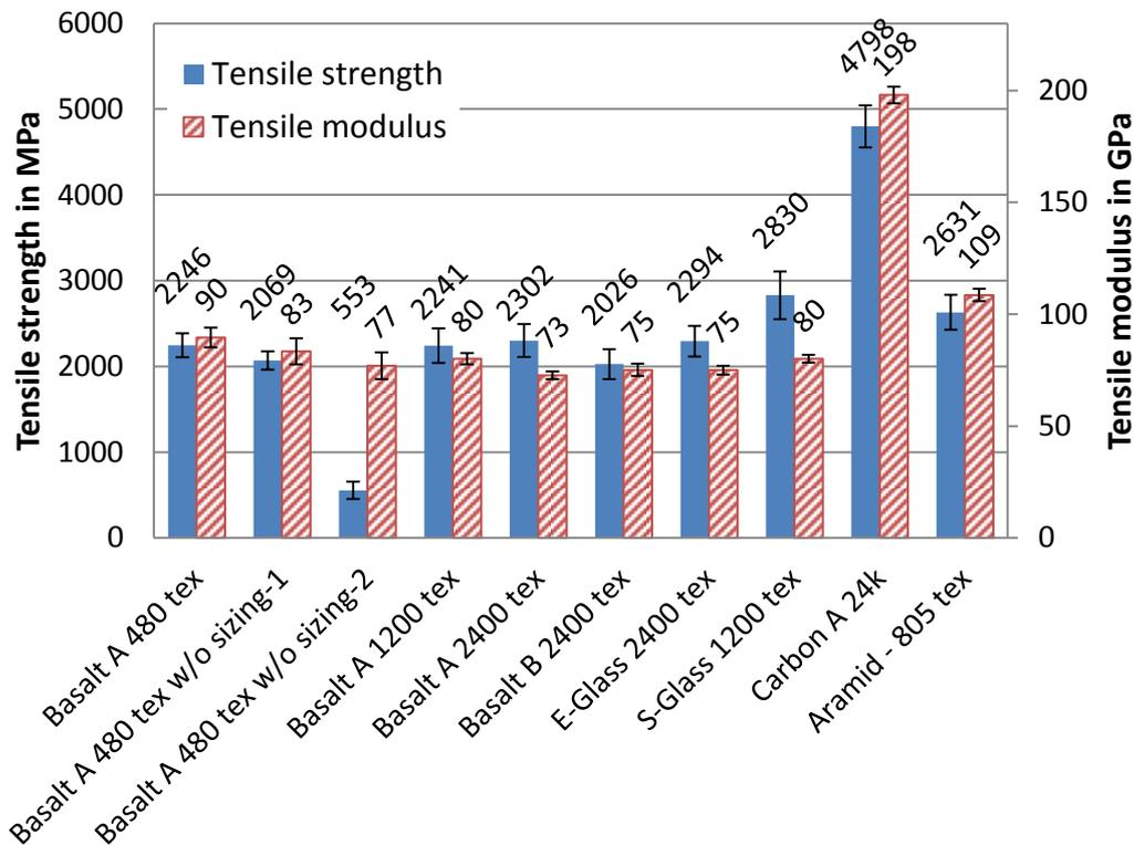
Figure 6: Tensile properties of impregnated roving specimens
