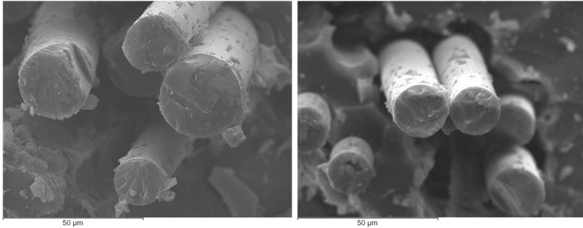
Figure 7: Scanning electron micrograph of fracture surfaces of impregnated basalt fiber roving (left) and glass fiber roving (right) after tensile test, both showing brittle glass fracture pattern
