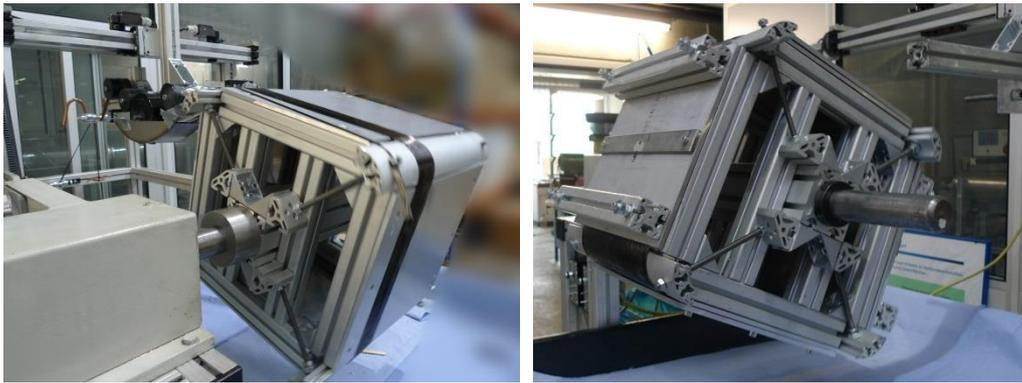
Figure 1: Filament winding of unidirectional plates – left: winding mandrel for flat composite plates; right: attachment of stiffening plates
