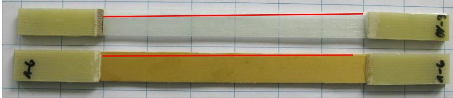
Figure 12: Single fracture in E-glass- and aramid-tensile test specimens at +23 °C, which led to stop of test apparatus; test specimens were tested again until final failure afterwards
