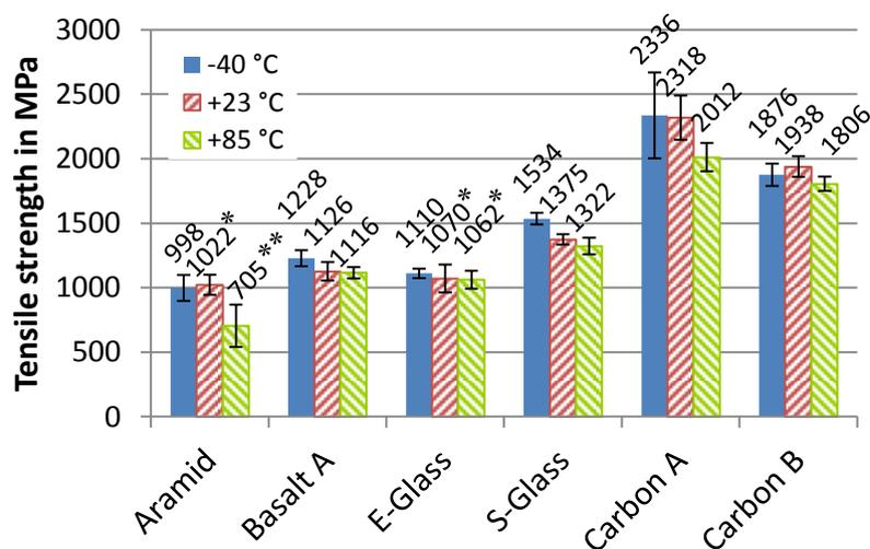
Figure 8: Tensile strength of different tested polymer fiber composites with epoxy matrix at -40 °C, +23 °C and +85 °C (\* - test restarted at +23 °C after initial crack led to stop of testing machine; \*\* - invalid result, failure only by debonding of cap strips)
