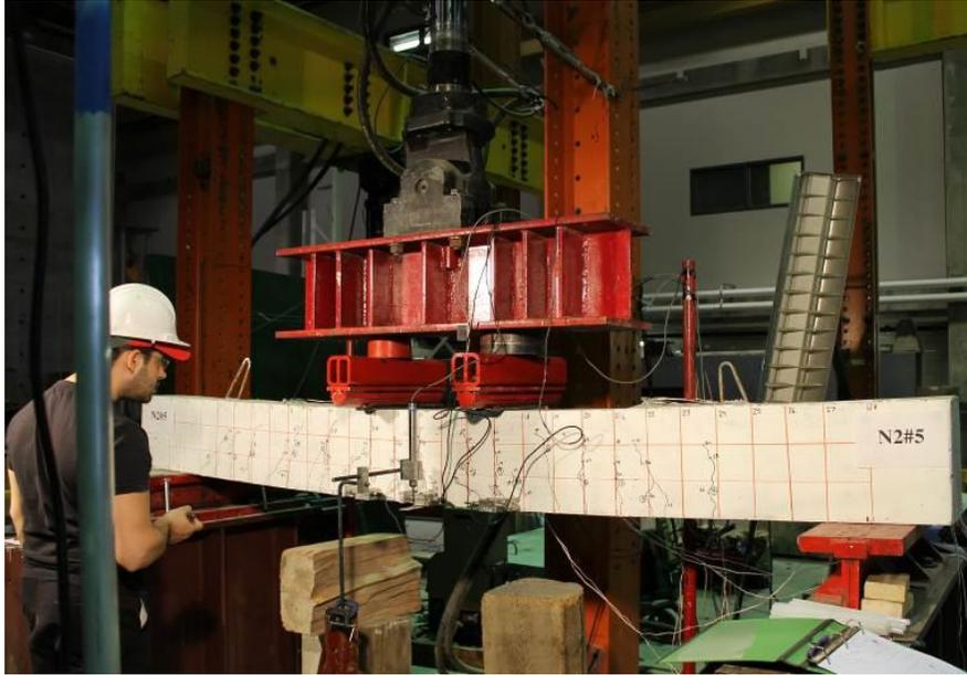
Figure 6: Test setup during a beam test
