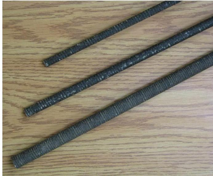
Figure 1: Basalt FRP bars
